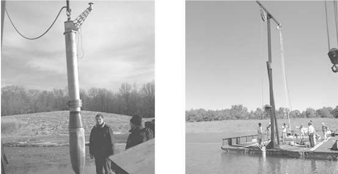
Figure 3-3: The prototype flow shield and pressure case and the test rig at the Briar Point Test Facility.
